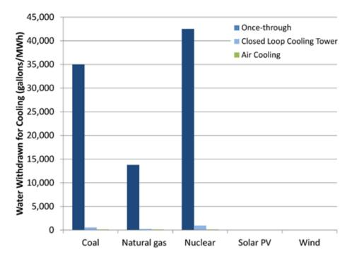
Figure 1. Comparison of Water Withdrawals by Various Cooling Technologies and Fuels<sup>94</sup>
