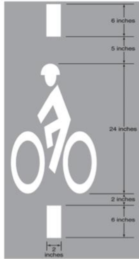
Figure 4-2 Bicycle Detector Pavement Marking
