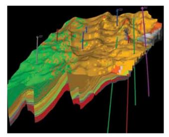
Using the results of appraisal wells and 3-D seismic, engineers and geoscientists build **computer simulations** of reservoirs to maximize recovery of oil and natural gas by better understanding the best locations to drill wells.
