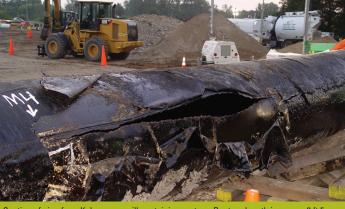
Section of pipe from Kalamazoo spill containing rupture. Rupture length is approx 6 ft 5 inches and is 4 1/2 inches wide at the widest location.
