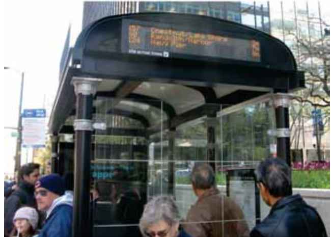
FIGURE 54 LED DMS in CTA bus shelter outside 222 South Riverside Plaza (Courtesy: David Phillips 2012).
