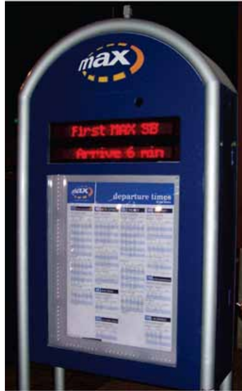
FIGURE 25 KCATA MAX (BRT service) DMS (Courtesy: TranSystems 2005).
