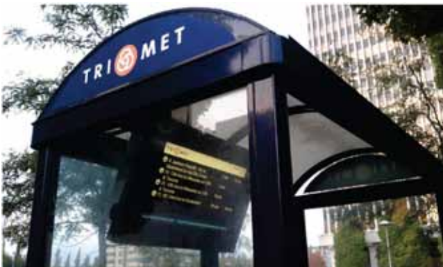
FIGURE 48 TriMet LCD DMS at bus stop near Lloyd Center (Courtesy: Carol Schweiger 2011).
