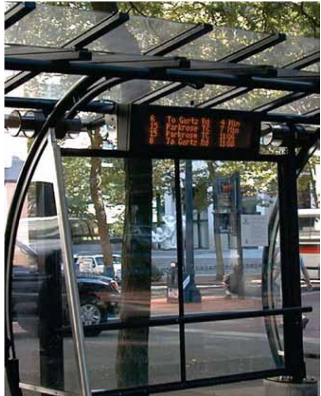
FIGURE 45 Dynamic message sign in TriMet bus shelter.
