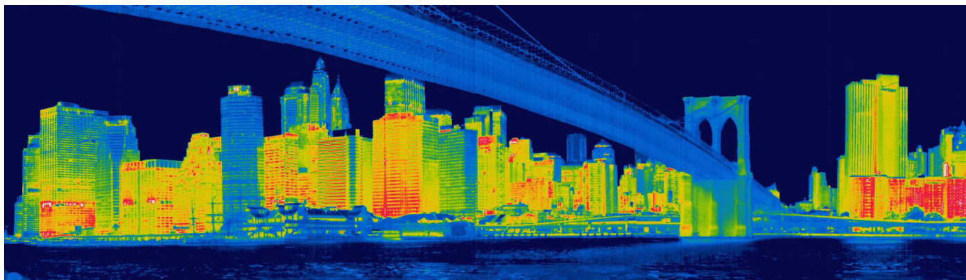
Figure 1.2: Infrared image showing heat loss from New York City buildings
