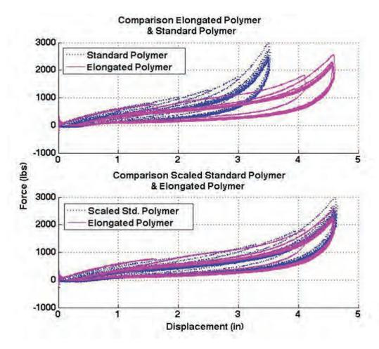
*Comparison between mechanical response of a standard length and modified length polymer equidistant device*
