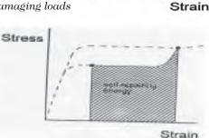
(b) Self-repair using the absorbed energy
