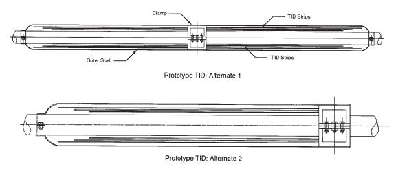
**Figure 1** *Tuned Induced Damper (TID) system.*
