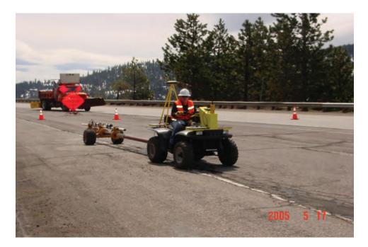
**Figure 1** *Mobile geophysical subsurface scoping equipment.*
