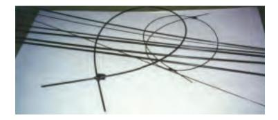
**Figure 1** Basalt fiber composite rebars.
