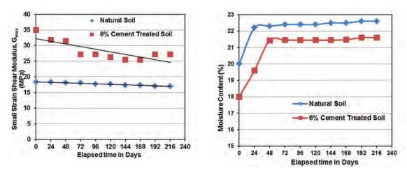
Shear modulus and moisture content variation with elapsed time period of Oklahoma soil specimens (sulfate content of 15,200 ppm).
