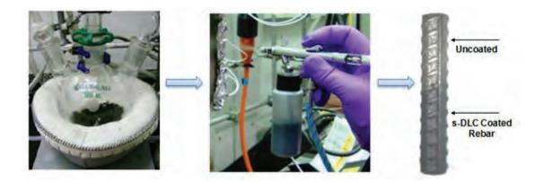
Developed atmospheric solution-based processing technology by which DLC coatings can be deposited on carbon steel coupons and rebar samples. Process steps involve chemical synthesis of DLC polymer precursors, spray-coating polymer precursor solutions onto steel substrates, and subsequent heat treatment to convert films to s-DLC.
