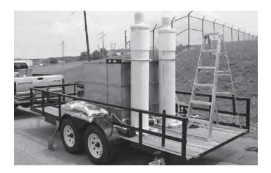
Figure 1 Wash water filtration system.
