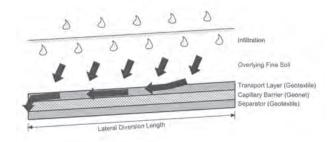
**Figure 1** *Geocomposite capillary barrier drain.*
