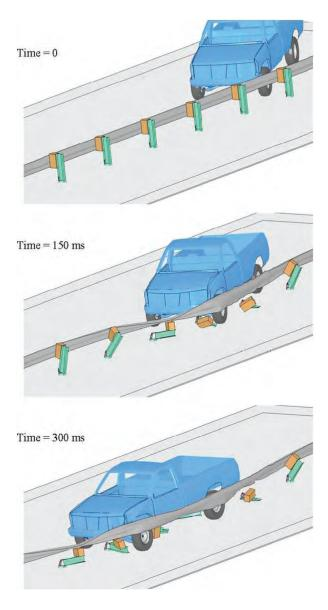
Simulation of crash test of W-beam guardrail system with energy absorbing breakaway posts.
