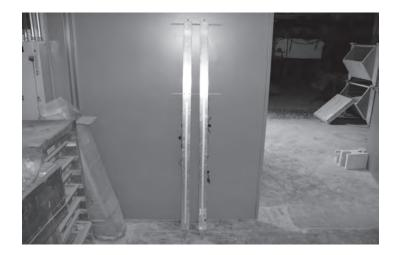
**Figure 1** *The cone penetrometer equipped with piezoelectric sensors.*
