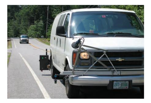
Figure 1 Prototype Retroreflectivity Mobile Unit. mance requirements of accuracy, repeatability, and reproducibility. A simple daily verification procedure will be used in place of the hourly calibration required of the existing systems. Only a single operator will be required as opposed to two needed to operate the existing technology. Potentially, the system could simultaneously measure two lanes instead of one.
