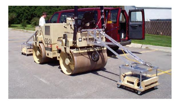
**Figure 1** *Prototype system for asphalt pavement density determination.*
