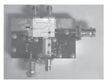
**Figure 1** *The millimeter-wave sensor prototype.*
