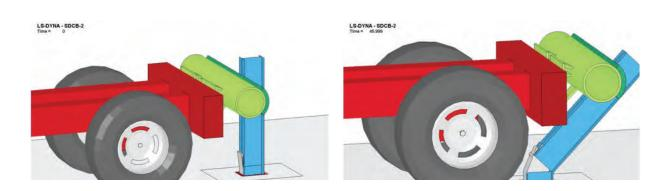
**Figure 3** *Illustration of failure mechanism for bent plate design.*
