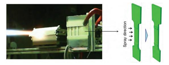
Photograph of the test sample preparation and illustrative schematic of tensile testing strategy. The image on the left is the thermal spray plume impacting the in-situ-coating-property sensor, which allows for determination of residual stresses and coating properties through beam curvature measurements. The image on the right displays grooved or ungrooved dog bones that were used to conduct testing of simulated reclamation process.
