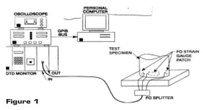
Fiber-optic sensor data acquisition system.
