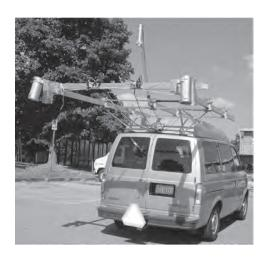
Figure 1 The dual-camera subsystem.
