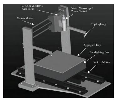
Figure 1 3-D graphical model of AIMS.
