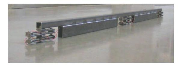
**Figure 1** *Photograph of weigh-in-motion sensor.*
