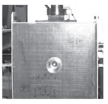
Figure 2 Photo of FRP panel and connector.
