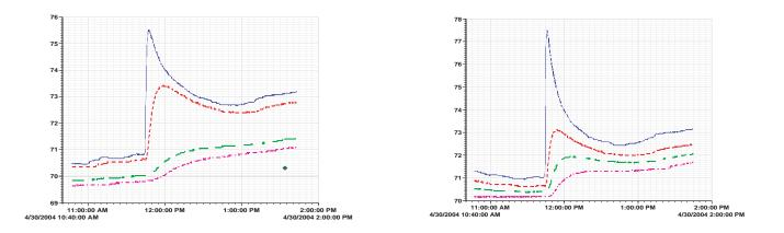
**Figure 1** *Temperature profiles: (left) at delamination and (right) in sound area at various sensor depths.*
