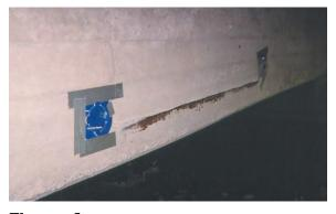
Figure 1 Installed optical sensor.
