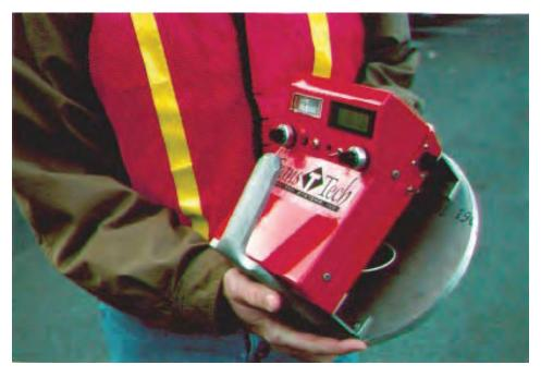
**Figure 1** Advanced prototype of TransTech System's pavement quality indicator.
