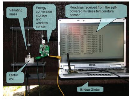
**Figure 1** Prototype of the self-powered wireless sensor.
