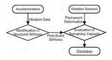
Figure 1 Proposed damage assessment and capacity estimation method.
