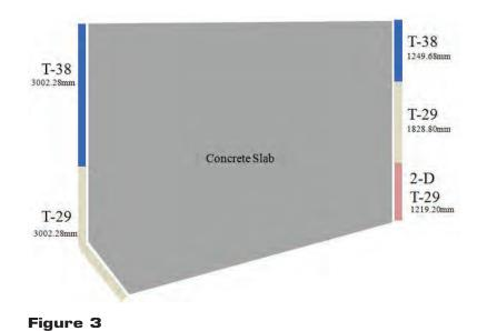
A schematic of installed sealant in expansion joint (T-38: glass transition temperature of 38°C; T-29: glass transition temperature of 29°C; 2-D: two-dimensional programming).
