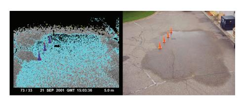
**Figure 2** *Areas of wet and dry pavement can be detected by the system.*
