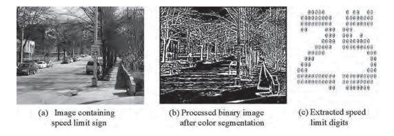
Figure 1 Speed limit sign extraction.
