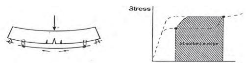
(a) Superelastic energy absorption under damaging loads
