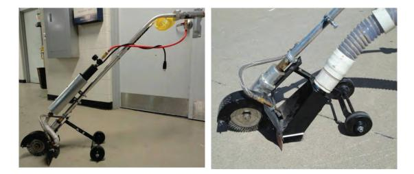
**Figure 1** *Heat lance configuration (left) and vacuum configuration (right).*
