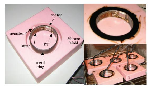
**Figure 1** *ABCD ring in a silicone mold (left); binder specimens prepared for ABCD test (right).*
