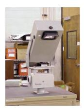
**Figure 1** *Prototype ice detection system.*
