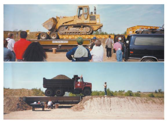
**Figure 1** *Composite bridge under test in Russell, Kansas.*
