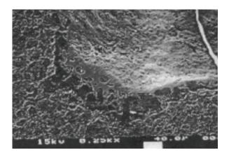
**Figure 1** Scanning electron micrograph of coating prepared by paint-and-heat metallization.
