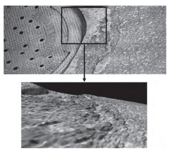
**Figure 1** *Visualization of 3-D pavement surface data for analyzing loss of stones.*
