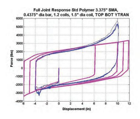
**Figure 3** *Full joint behavior incorporating in series polymer SMA configuration.*
