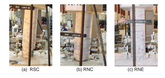
**Figure 1** *Residual displacement and damage after 10 percent maximum drift.*
