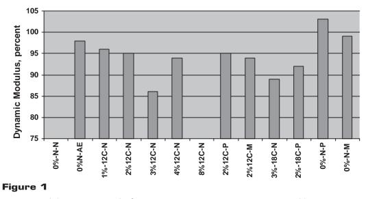
Freezing and thawing test results for concrete specimens containing organic additives.
