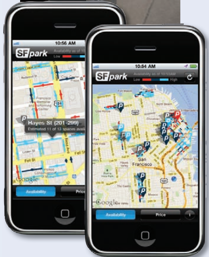
San Francisco's SFpark parking management system uses sensors to adjust meter prices based on demand. Users can access information with smartphones. (Photo courtesy SFpark)
