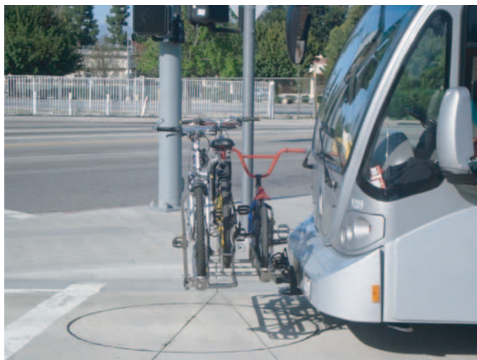
Exhibit 8-6. Exterior bicycle rack on BRT vehicle (Los Angeles).
