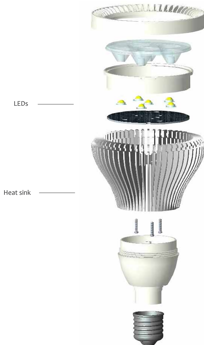
LED example assembly for thermal management
