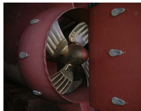
Figure 3.11 Nozzles Enclosing Propeller to Reduce Friction Losses
